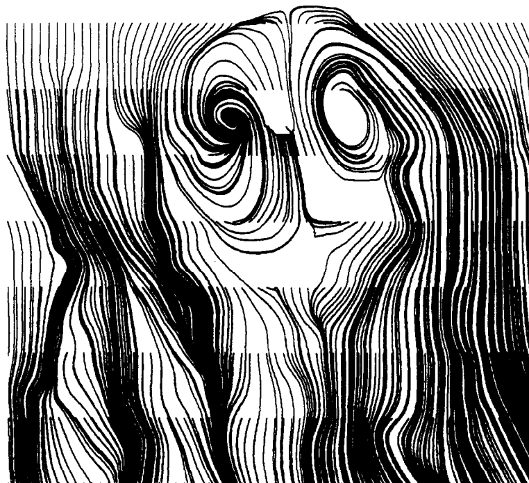
Figure 20. Particle trace based on the interpolated velocities of figure 17. Gas bubble in mineral oil. Experiment 89.
